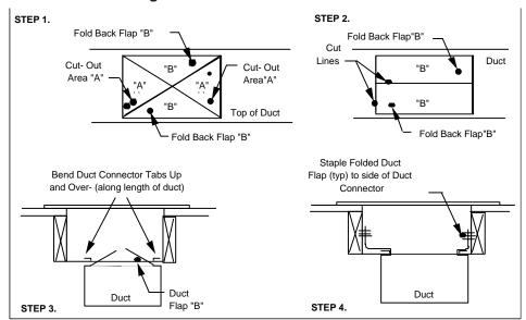
Figure 12. Alternate Installation
